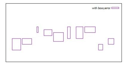
The **boxxyerror** plot style is only relevant to 2D data plotting. It is similar to the <u>xyerrorbars</u> style except that it draws rectangular areas rather than crosses. It uses either 4 or 6 basic columns of input data. Additional input columns may be used to provide information such as variable line or fill color (see <u>rgbcolor variable</u>).
