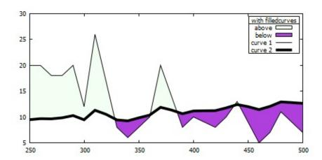
The **filledcurves** style is only used for 2D plotting. It has three variants. The first two variants require either a single function or two columns (x,y) of input data, and may be further modified by the options listed below.
