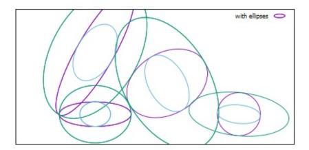
The **ellipses** style plots an ellipse at each data point. This style is only relevant for 2D plotting. Each ellipse is described in terms of its center, major and minor diameters, and the angle between its major diameter and the x axis.
