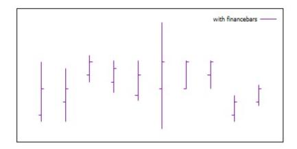
The symbol is a vertical line segment, located horizontally at the x coordinate and limited vertically by the high and low prices. A horizontal tic on the left marks the opening price and one on the right marks the closing price. The length of these tics may be changed by <u>set errorbars</u>. The symbol will be unchanged if the high and low prices are interchanged. See <u>set errorbars</u> and <u>candlesticks</u>, and also the <u>finance demo</u>.
