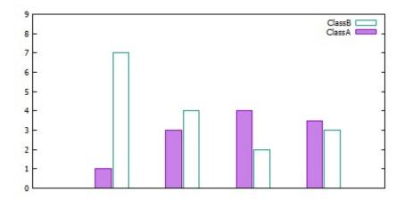
Suppose that the input file contains data values in columns 2, 4, 6, ... and error estimates in columns 3, 5, 7, ... This example plots the values in columns 2 and 4 as a histogram of clustered boxes (the default style). Because we use iteration in the plot command, any number of data columns can be handled in a single command. See plot for.
