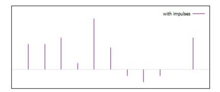
The **impulses** style displays a vertical line from y=0 to the y value of each point (2D) or from z=0 to the z value of each point (3D). Note that the y or z values may be negative. Data from additional columns can be used to control the color of each impulse. To use this style effectively in 3D plots, it is useful to choose thick lines (linewidth > 1). This approximates a 3D bar chart.
