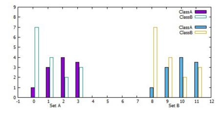
The **at** <**x-coord**> option sets the x coordinate position of the following histogram to <x-coord>. For example
