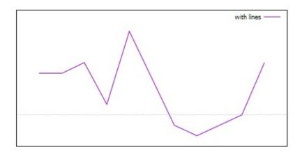
The **lines** style connects adjacent points with straight line segments. It may be used in either 2D or 3D plots. The basic form requires 1, 2, or 3 columns of input data. Additional input columns may be used to provide information such as variable line color (see <u>rgbcolor variable</u>).
