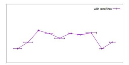
The **xerrorlines** style is only relevant to 2D data plots. **xerrorlines** is like linespoints, except that a horizontal error line is also drawn. At each point (x,y), a line is drawn from (xlow,y) to (xhigh,y) or from (x-xdelta,y) to (x+xdelta,y), depending on how many data columns are provided. The appearance of the tic mark at the ends of the bar is controlled by <u>set errorbars</u>. The basic style requires either 3 or 4 columns:
