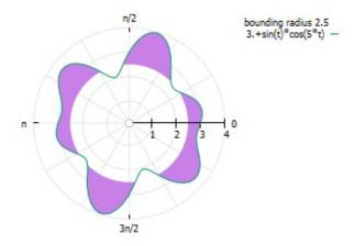
Polar plots are generated by changing the current coordinate system to polar before issuing a plot command. The option <u>set polar</u> tells gnuplot to interpret input 2D coordinates as <angle>,<radius> rather than <x>,<y>. Many, but not all, of the 2D plotting styles work in polar mode. The figure shows a combination of plot styles <u>lines</u> and <u>filledcurves</u>. See <u>set polar</u>, <u>set rrange</u>, <u>set size square</u>, <u>set theta</u>, <u>set ttics</u>.
