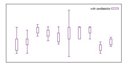
The **candlesticks** style can be used for 2D data plotting of financial data or for generating box-and-whisker plots of statistical data. The symbol is a rectangular box, centered horizontally at the x coordinate and limited vertically by the opening and closing prices. A vertical line segment at the x coordinate extends up from the top of the rectangle to the high price and another down to the low. The vertical line will be unchanged if the low and high prices are interchanged.
