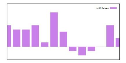
The width of the box is obtained in one of three ways. If the input data has a third column, this will be used to set the width of the box. If not, if a width has been set using the <u>set boxwidth</u> command, this will be used. If neither of these is available, the width of each box will be calculated automatically so that it touches the adjacent boxes.
