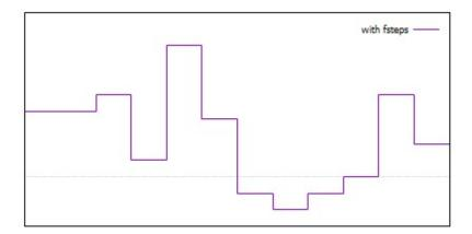
The **fsteps** style is only relevant to 2D plotting. It connects consecutive points with two line segments: the first from (x1,y1) to (x1,y2) and the second from (x1,y2) to (x2,y2). The input column requires are the same as for plot styles <u>lines</u> and <u>points</u>. The difference between **fsteps** and <u>steps</u> is that **fsteps** traces first the change in y and then the change in x. <u>steps</u> traces first the change in y.
