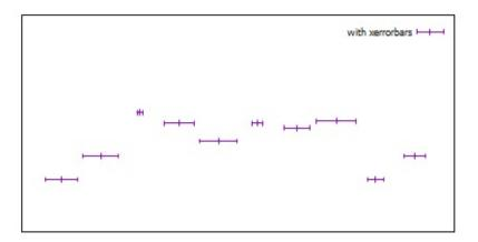
The **xerrorbars** style is only relevant to 2D data plots. **xerrorbars** is like <u>points</u>, except that a horizontal error bar is also drawn. At each point (x,y), a line is drawn from (xlow,y) to (xhigh,y) or from (x-xdelta,y) to (x+xdelta,y), depending on how many data columns are provided. The appearance of the tic mark at the ends of the bar is controlled by <u>set errorbars</u>. The basic style requires either 3 or 4 columns:
