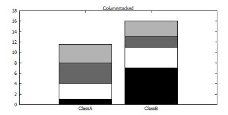
will produce two vertical stacks, one for each column of data. The stack at x=1 will contain a box for each entry in column 2 of the datafile. The stack at x=2 will contain a box for each parallel entry in column 4 of the datafile.
