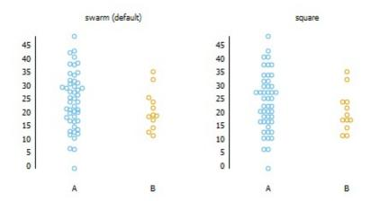
"Bee swarm" plots result from applying jitter to separate overlapping points. A typical use is to compare the distribution of y values exhibited by two or more categories of points, where the category determines the x coordinate. See the <u>set jitter</u> command for how to control the overlap criteria and the displacement pattern used for jittering. The plots in the figure were created by the same plot command but different jitter settings.
