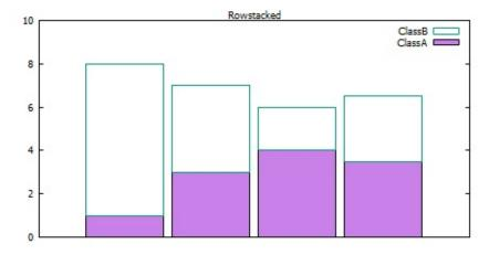
This will produce a plot in which each vertical bar corresponds to one row of data. Each vertical bar contains a stack of two segments, corresponding in height to the values found in columns 2 and 4 of the datafile.
