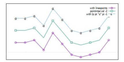
The **linespoints** style (short form **lp**) connects adjacent points with straight line segments and then goes back to draw a small symbol at each point. Points are drawn with the default size determined by <u>set pointsize</u> unless a specific point size is given in the plot command or a variable point size is provided in an additional column of input data. Additional input columns may also be used to provide information such as variable line color. See <u>lines</u> and <u>points</u>.
