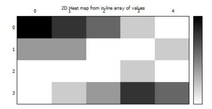
This figure illustrates generation of a heat map from an array of scalar values. The current palette is used to map each value onto the color assigned to the corresponding pixel.
