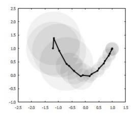
The **circles** style plots a circle with an explicit radius at each data point. If three columns of data are present, they are interpreted as x, y, radius. The radius is always interpreted in the units of the plot's horizontal axis (x or x2). The scale on y and the aspect ratio of the plot are both ignored. If only two columns are present, the radius is taken from <u>set style circle</u>. In this case the radius may be given in graph or screen coordinates.
