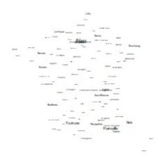
The **labels** style reads coordinates and text from a data file and places the text string at the corresponding 2D or 3D position. 3 or 4 input columns of basic data are required. Additional input columns may be used to provide properties that vary point by point such as text rotation angle (keywords **rotate variable**) or color (see <u>textcolor variable</u>).
