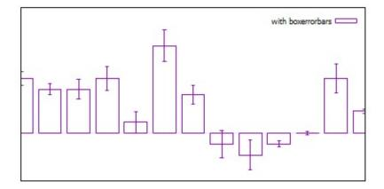
The boxwidth will come from the fourth column if the y errors are given as "ydelta" and the boxwidth was not previously set to -2.0 (**set boxwidth -2.0**) or from the fifth column if the y errors are in the form of "ylow yhigh". The special case **boxwidth = -2.0** is for four-column data with y errors in the form "ylow yhigh". In this case the boxwidth will be calculated so that each box touches the adjacent boxes. The width will also be calculated in cases where three-column data are used.
