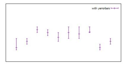
The **yerrorbars** (or <u>errorbars</u>) style is only relevant to 2D data plots. **yerrorbars** is like <u>points</u>, except that a vertical error bar is also drawn. At each point (x,y), a line is drawn from (x,y)-ydelta to (x,y)-ydelta or from (x,y)-ydelta to (x,y)-ydelta or from (x,y)-ydelta, to (x,y)-ydelta or from (x,y)-ydelta or fro
