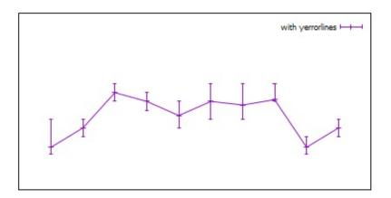
The **yerrorlines** (or <u>errorlines</u>) style is only relevant to 2D data plots. **yerrorlines** is like <u>linespoints</u>, except that a vertical error line is also drawn. At each point (x,y), a line is drawn from (x,y)-ydelta) to (x,y)+ydelta) or from (x,y)-by to (x,y)-high), depending on how many data columns are provided. The appearance of the tic mark at the ends of the bar is controlled by <u>set errorbars</u>. Either 3 or 4 input columns are required.
