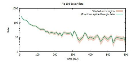
The third variant fills the area between two curves sampled at the same set of x coordinates. It requires three columns of input data (x, y1, y2). This is the default if there are three or more columns of input data. If you have a y value in column 2 and an associated error value in column 3 the area of uncertainty can be represented by shading. See also the similar 3D plot style zerrorfill.
