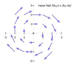
The 2D **vectors** style draws a vector from (x,y) to (x+xdelta,y+ydelta). The 3D **vectors** style is similar, but requires six columns of basic data. In both cases, an additional input column (5th in 2D, 7th in 3D) may be used to provide variable (per-datapoint) color information. (see <u>linecolor</u> and <u>rgbcolor variable</u>). A small arrowhead is drawn at the end of each vector.
