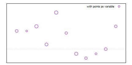
The **points** style displays a small symbol at each point. The command **set pointsize** may be used to change the default size of the points. The point type defaults to that of the linetype. See <u>linetype</u>. If no <u>using</u> spec is found in the plot command, input data columns are interpreted implicitly. See <u>style lines</u>.
