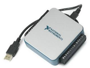
It provides 4 analogue inputs, 2 analogue voltage outputs and 8 TTL digital outputs (with limited functionality). Analogue sampling/timing intervals are limited to  $\geq 0.2$ ms. TTL digital outputs are updated no faster than at 50 ms intervals and are not accurately synchronised with camera exposures, preventing their use for the control of multi-
