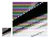
A regular slant to a decoded image with rainbows across scanlines is usually indicative of a buggy video codec that does not compute *pitch* or *stride* correctly. The technical reason for this is that padding at the end of each horizontal row is not being accounted for correctly, resulting in each row being progressively further off. This isn't that important to diagnose the problem, though.
