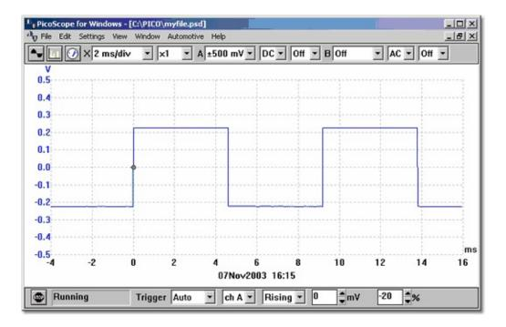
If the trigger event occurs only once, it is useful to be able to stop immediately after collecting the data for the trigger event. You can do this by checking the
