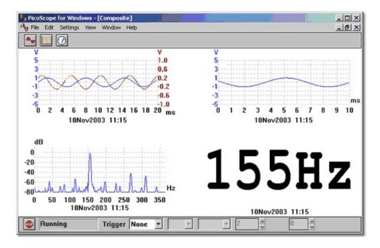
You can control what combination of window data is displayed in the composite window, and in what order it is displayed. The following options - accessed from the Layout drop-down list in the Options... menu in Settings - are available for the composite window:
