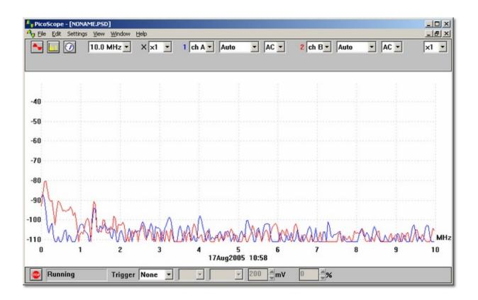
The spectrum analyser window uses a **FFT** to convert a set of samples taken at fixed time intervals into a distribution showing the amount of energy in each of a number of frequency bands up to a maximum frequency. The maximum frequency is half the frequency corresponding to the sampling rate.
