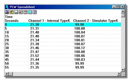
There is one line for each reading. The first column shows the time in seconds, while the remaining columns show the selected measurements.
