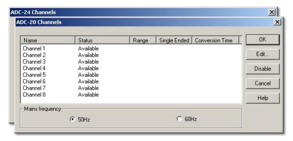
**Status.** If an even-numbered analog channel is being used in conjunction with its corresponding odd-numbered channel to form a differential input pair, its status will be shown as 'Unavailable'.
