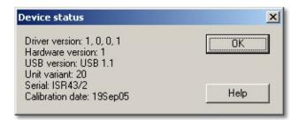
This dialog box displays the details about the <u>ADC</u> connection to the computer.
