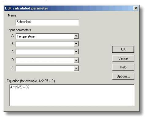
This dialog box enables you to edit the details for a calculated measurement. A calculated measurement is calculated from up to five other measurements, using an equation.
