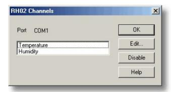
This dialog box is used to select the channels that will be used to take measurements.
