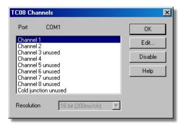
This dialog box is used to select the channels that will be used to take measurements.
