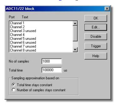
This dialog box is used to select the channels and sampling rate for fast recording.
