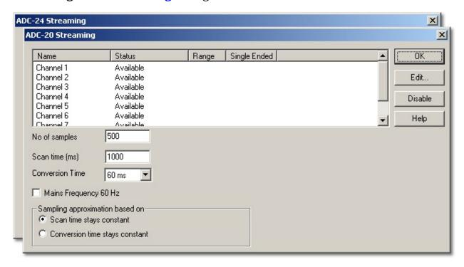
**Edit.** To edit a channel, highlight it and click the **Edit** button. This will open the **Edit ADC-20 Streaming Channel** or **Edit ADC-24 Streaming Channel** dialog box so that you can enter the details.
