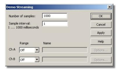
This dialog box only applies to the block method of recording. It is used to select the channels that will be used to take measurements.
