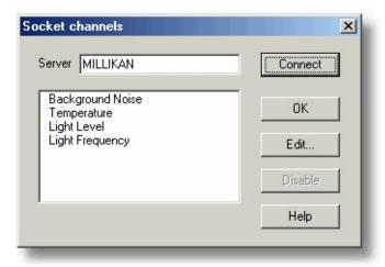
This dialog box is used to establish a connection to another instance of PicoLog running on a remote <u>server</u> computer, and then to select the channels that are to be imported to this instance of PicoLog.
