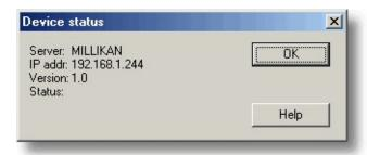
This dialog box displays the details about the <u>IP socket</u> connection to the <u>server</u>.
