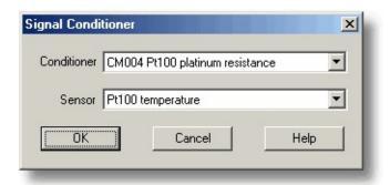
This dialog box provides support for the Pico range of signal conditioners. A signal conditioner provides excitation or power, or both, for a sensor and then amplifies the output from the sensor.
