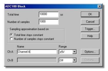
This dialog box only applies to the block method of recording. It is used to select the channels that will be used to take measurements.
