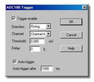
Triggering is used to select the moment at which PicoLog collects data - usually at some fixed time before or after a trigger event.
