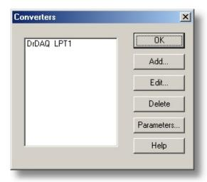
This dialog box is used to build up a list of <u>converters</u> to use. In the pane on the left will be a list of the converters that are currently active.
