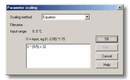
This dialog box is used to specify how to convert a measurement value into some other unit, for example from volts to temperature. It is invoked when you click the **Scaling** button in the **Parameter options** dialog box.
