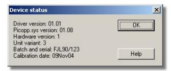
This dialog box displays details of the ADC status. The calibration date will help you keep track of when the unit should be returned to Pico for optional annual recalibration.
