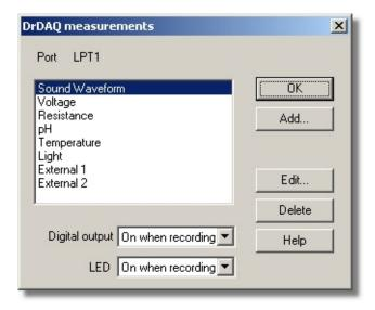
This dialog box is used to build up a list of measurements to measure for a converter. On the left is the current list of measurements and on the right are buttons to update the list.
