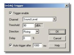
Triggering is used to select the moment at which PicoLog starts collects data - usually at some fixed time before or after a trigger event.
