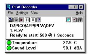
At the top is a menu bar containing the <u>File</u>, <u>Settings</u>, <u>View</u> and <u>Help</u> menus. Below the menu bar are two sets of controls, the Recorder controls and the Window controls.
