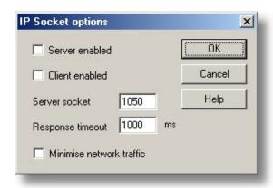
This dialog box is used to specify the details required to establish a link between computers via an IP network.
