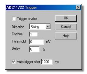
Triggering is used to select the moment at which PicoLog starts collects data - usually at some fixed time before or after a trigger event.
