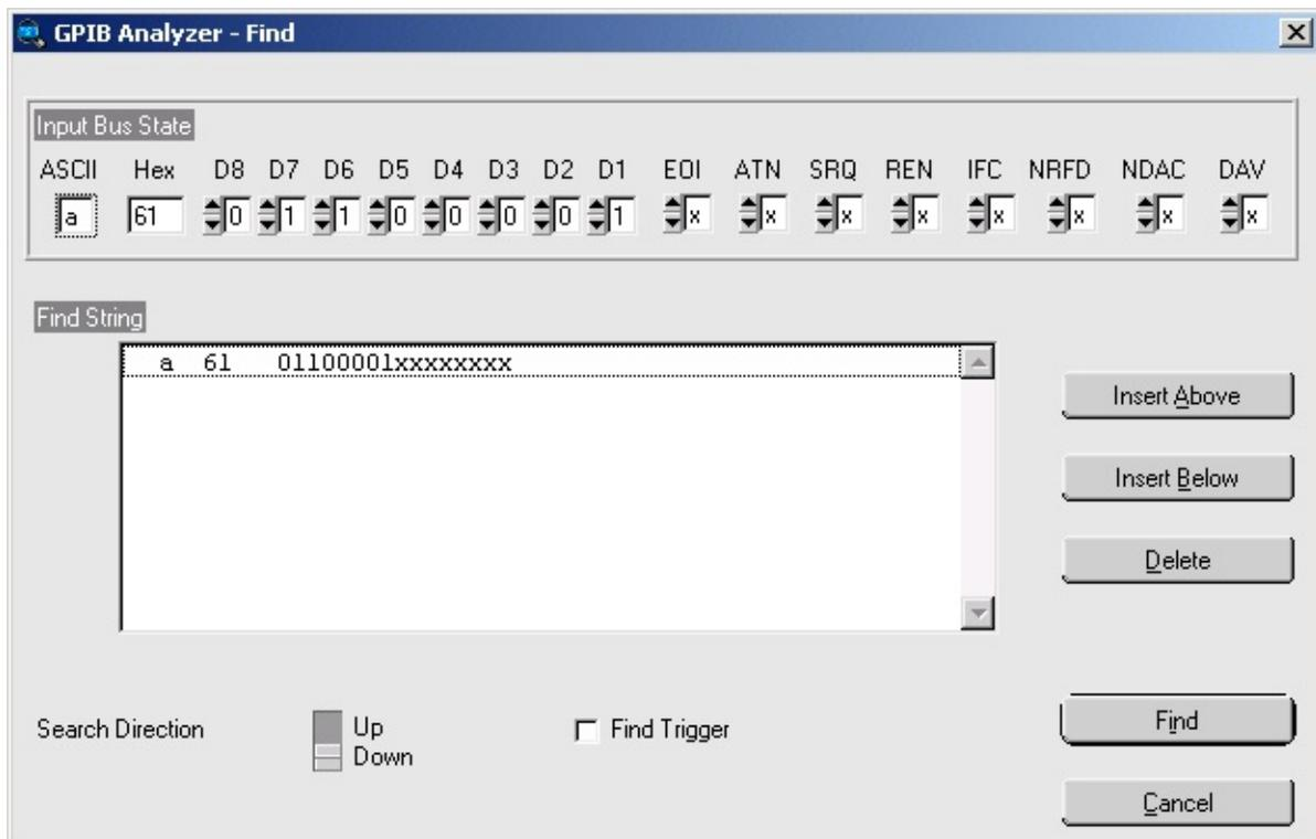
To find a trigger point in the Capture Display window, check the **Find Trigger** checkbox and then click the **Find** button.
