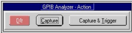
Note that you can switch back and forth between [Capture](#) and [Capture & Trigger](#) during the capture without losing data.
