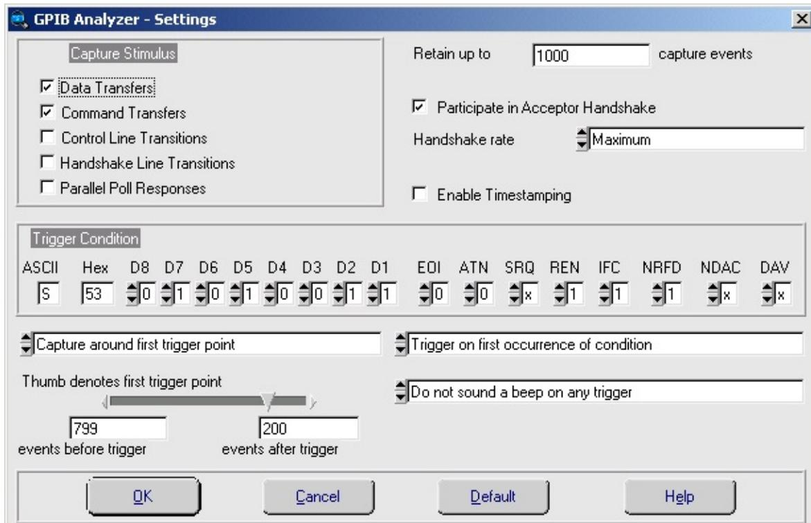
The configured settings apply only to active capture displays. Note that the settings in this window cannot be changed unless capturing and triggering are turned off (use the [Action](#) window to turn off capturing and triggering).
