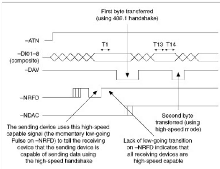
The following steps describe a typical sequence of events in an HS488 data transfer in which the Talker and Listener are both HS488 capable.
