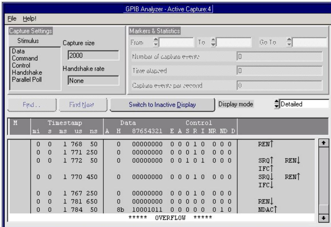
If an overflow error occurs, one or more GPIB events have been lost. You can usually avoid overflow errors by making one of the following changes:
