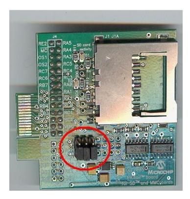
3. Insert the J2 slot of SD Card PICTail™ Plus Daughter Card into PICTail™ Plus (J8) port of PIC24FJ256DA210 development board with correct pin to pin mapping. Make sure that the SD Card Connector is facing away from the PIC24FJ256DA210 chip of the development board. Insert the SD Card in SD Card PICTail™ Plus Daughter board.
