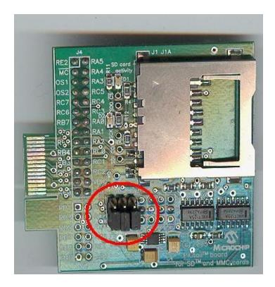
Insert the J4 port pins of SD Card PICTail™ Plus Daughter Card in the J3 port of PIC18 Explorer board with correct pin to pin mapping. Insert the SD Card in SD Card PICTail™ Plus Daughter board.
