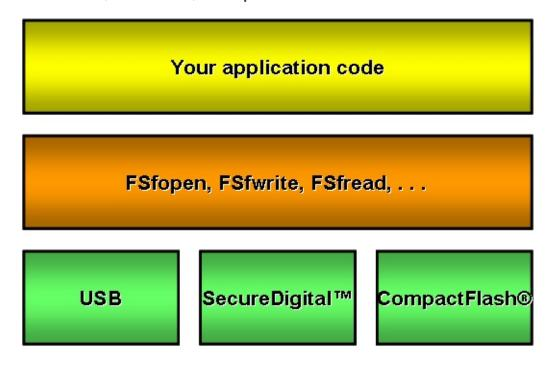
MDDFS supports all file and <u>directory</u> operations(like read,write,remove,rename...etc...). The maximum length of any file or <u>directory</u> name is restricted to 255 characters. The Long File Name(<u>LFN</u>) support is available for 16 and 32 bit PIC<sup>®</sup> microcontrollers. 8 bit PIC<sup>®</sup> MCU's doesn't support <u>LFN</u> feature due to comparatively lesser RAM size. Whereas the basic 8.3 format filename is supported by all 8, 16 & 32 bit PIC<sup>®</sup>
