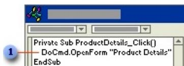
**1** The ProductDetails\_Click event procedure uses the **OpenForm** method to open the Product Details form.
