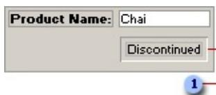
**1** This stand-alone toggle button is bound to the Discontinued field in the Products table. The button is pressed in, so the value in the field is **Yes**.
