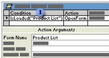
**1** This conditional expression uses the IsLoaded function to check whether the Product List form is open. The IsLoaded function is a sample [Function procedure](#) included with the Northwind sample database, and not a built-in Visual Basic function.
