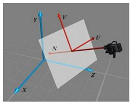
To transform the point **p**, multiply its homogeneous position vector ( $p_x$ ,  $p_y$ ,  $p_z$ , 1) by matrix *M*. The result is the transformed point in viewing coordinates. For pixel coordinates, you need to divide by the width and height of a pixel.
