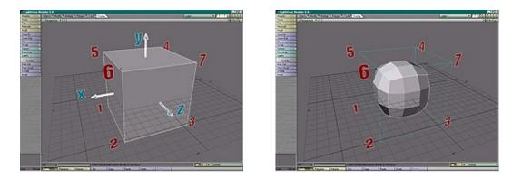
Loading the original cube (left) and activating subdivision patches turns the cube into a control cage for the patches (right). (The numbers in the figure are the point indexes. The hidden corner is point 0.) In the object file, the only difference between these two objects is the polygon type ID in the POLS chunk. For the subpatch version of the cube, the ID is PTCH rather than FACE.
