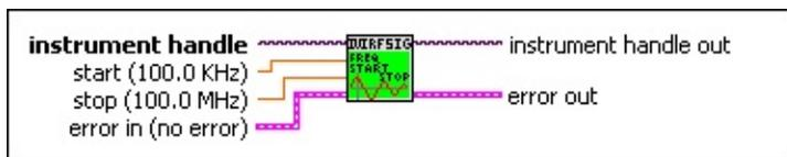
**I/O** **instrument handle** The instrument handle that you obtain from the [IviRFSigGen Initialize](#) or [IviRFSigGen Initialize With Options](#) VIs.
