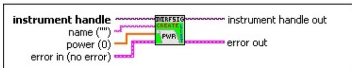
**I/O** **instrument handle** The instrument handle that you obtain from the [IviRFSigGen Initialize](#) or [IviRFSigGen Initialize With Options](#) VIs.
