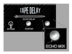
The *Echo Mix Knob* is a wet/dry balance control for the Tape Delay and dry AXXE/Drum signals, where positions less than 12 o'clock increase the amount of the dry signals, and positions greater than twelve o'clock increase the amount of the Tape Delay signal.
