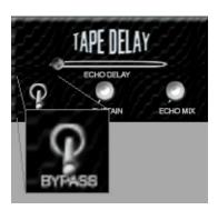
Click the *Bypass Switch* to enable or bypass the Tape Delay.
