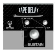
Move the *Sustain Knob* clockwise to increase the length of the echos, and counterclockwise to decrease the length of the echos.
