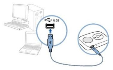
When the battery is charging, the Battery Level icon 💷 and Battery Charging icon 🔄 flash alternately on the player's display. The battery is fully charged when you see only the Charging Complete icon 🖘 on your player's display. If the display turns off automatically to save power, press any button to turn it on again.
