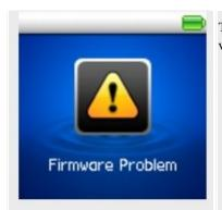
The firmware is corrupted. Reload the firmware, download a newer firmware version or contact Customer Support Services.
