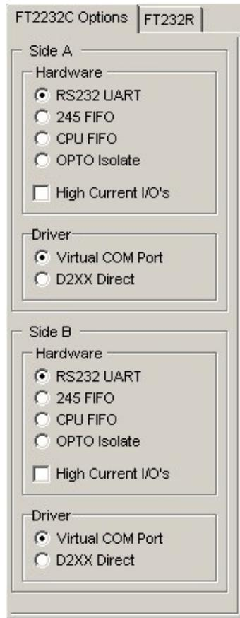
·Each channel can be independently configured as FT232BM-style USB UART or a FT245BM-style USB FIFO.
